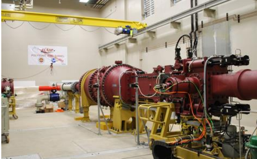
Figure 1 – FAMU-FSU polysonic wind tunnel capable of operation from Mach 0.2 to 5
